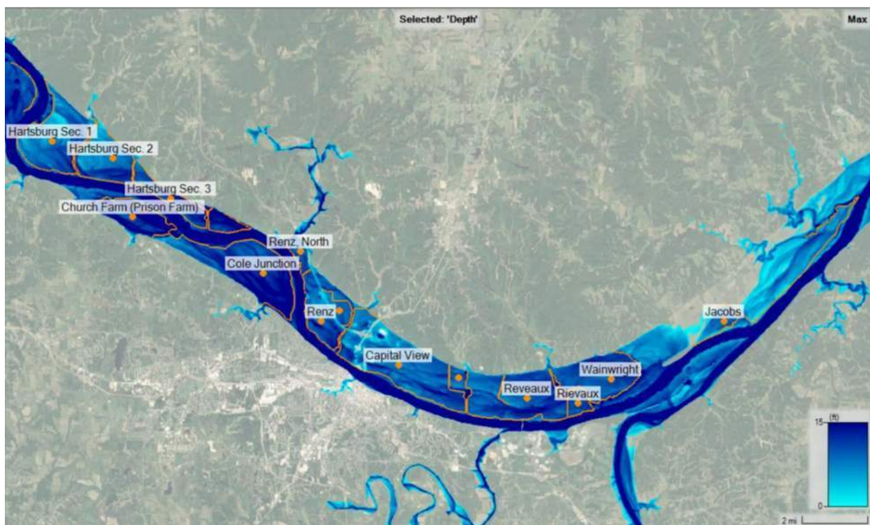
Figure 45. Inundation - CA0 - FWOP - 4% AEP
