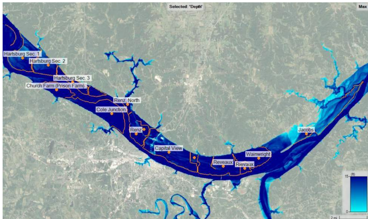
Figure 48. Inundation – CA0 - FWOP - 0.5% AEP
