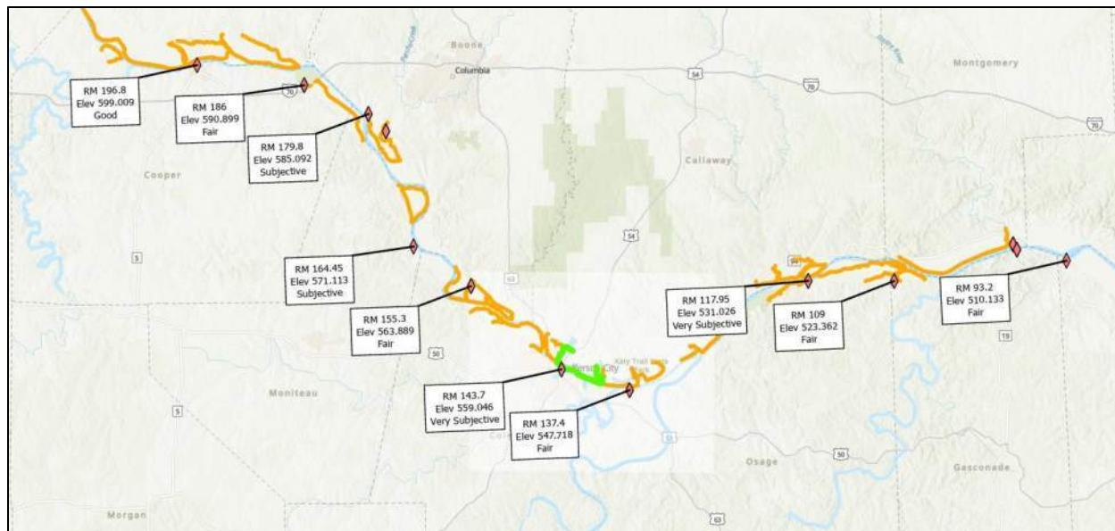
Figure 19. USACE Collected HWM for May 2019 Flood
