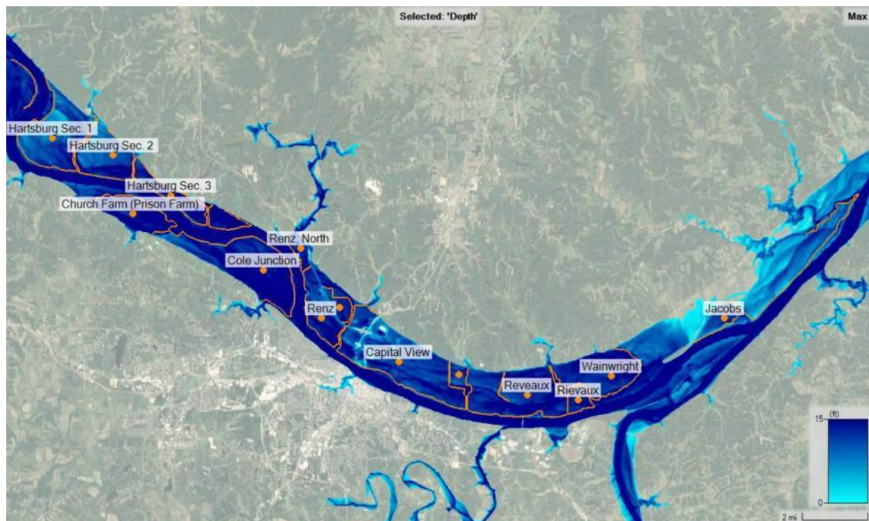
Figure 46. Inundation - CA0 - FWOP - 2% AEP
