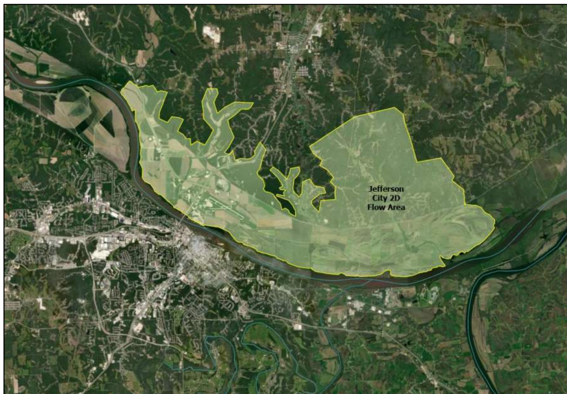
Figure 7. Jefferson City 2D Flow Area Delineation
